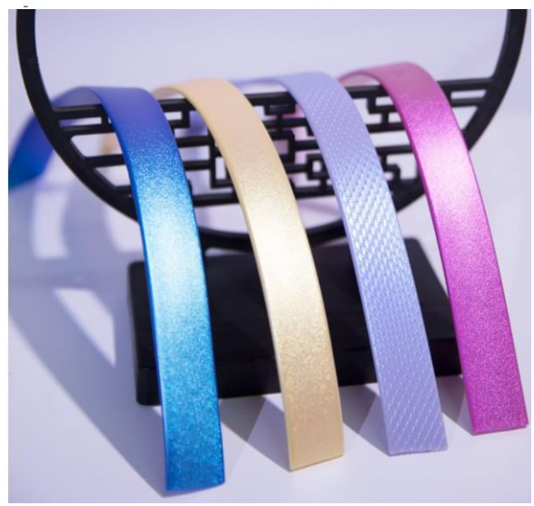
10)White nylon webbing+glittering PVC coating
